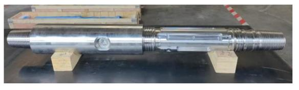
**Rotary Steerable drilling tool**
