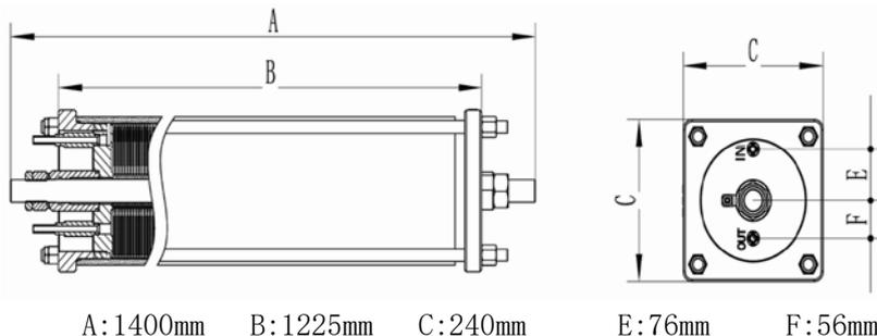
IN/OUT Interface diameter: 12mm      Water outlet: Quick hose connection 11.6x9
