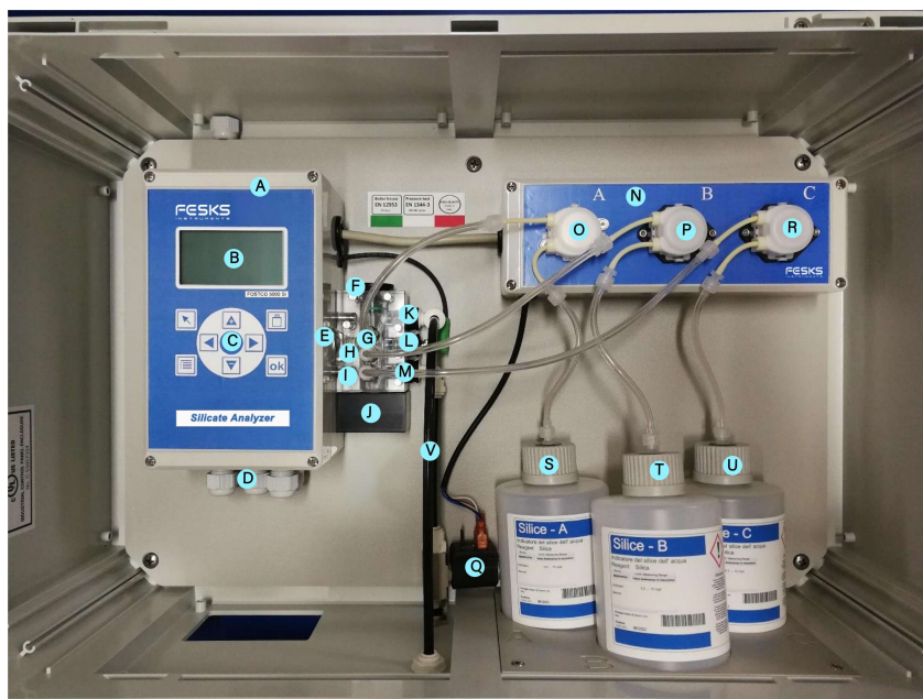
Illustration: DUROMAT® diamond SiO 2 analyzer with installed reagents.
