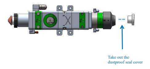
\* Align the red dot on the fiber optic head with the QBH red dot, and slowly insert the fiber optic head into the QBH.
