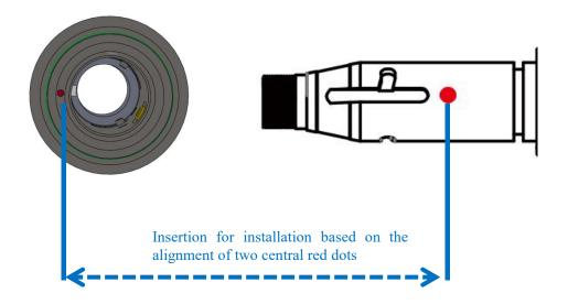
\* The QHB is screwed to the locking state: Rotate it to the limiting position clockwise (hearing the "click"), lift up the rotating mantle, and clockwise rotate the mantle until the head of optical fiber is compressed.
