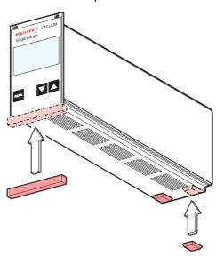
... and slip the supplied rubber bar onto the bottom edge of the front panel.
