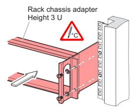
2 Slide the TPG 261 into the rack chassis adapter ...
