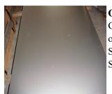
**GR23**: The material Gr23 is a modification alpha plus beta titanium alloy of Gr5, by reducing the content of intertitial elements, also named Gr5ELI. It offers improved toughness and resistance to low temperature.
