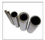
**GR12**: Alloyed with 3% aluminum and 2.5% vanadium gr12 titanium offers high resistance to pressure. The material has good ductility and toughness is widely used on bike frame. Cold-working and weldabilty are better than Gr5. Size: Dia0.2mm - 8mm \* WT0.015mm - 0.5mm \* L
