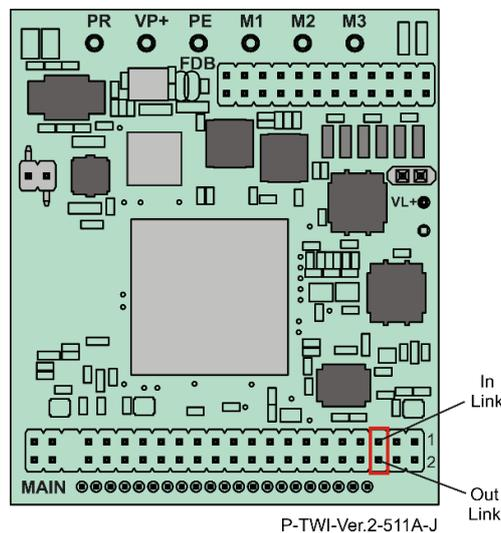
Figure 35: EtherCAT Link In and Out Pins
