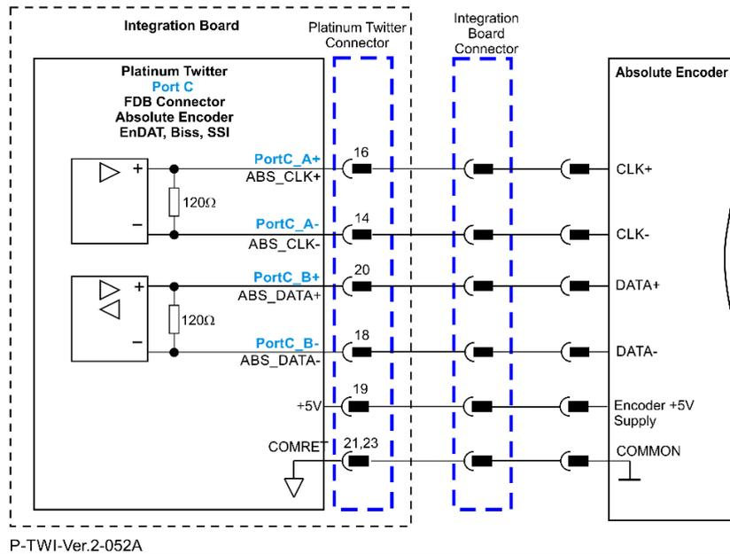
Figure 19: Absolute Serial Encoder – Recommended Connection Diagram for Endat, Biss, SSI
