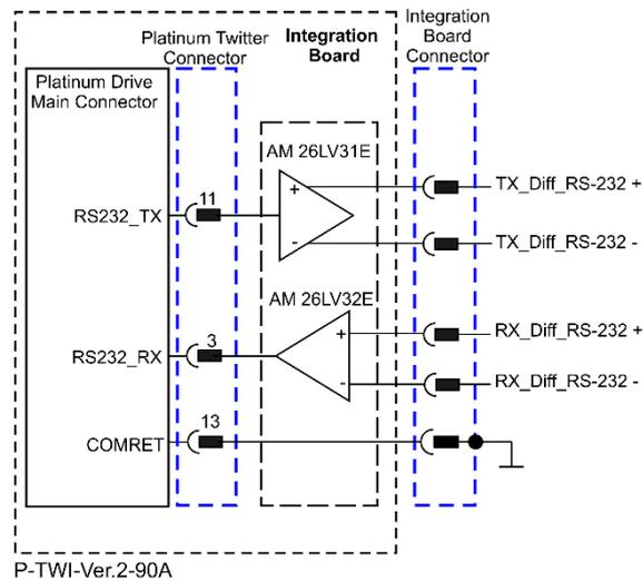
Figure 31: Differential RS232 (RS422) Connection Diagram
