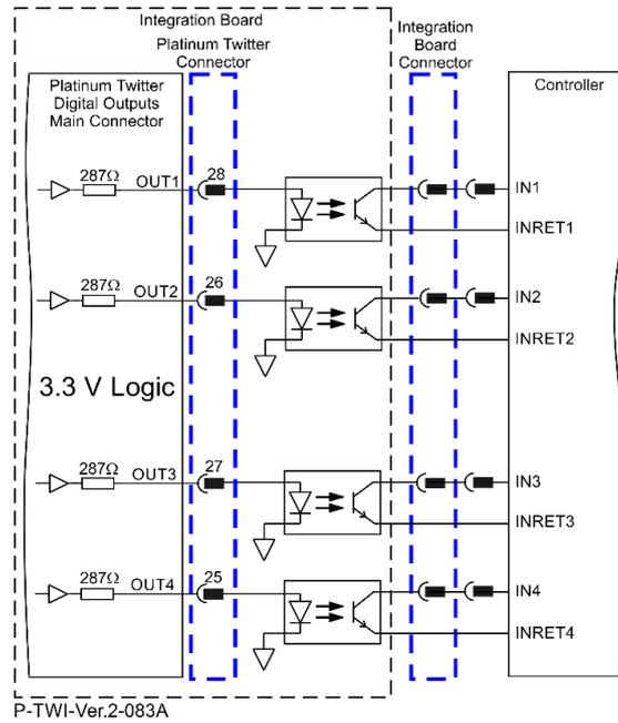
Figure 24: Digital Output 3.3V Logic Mode Connection Diagram
