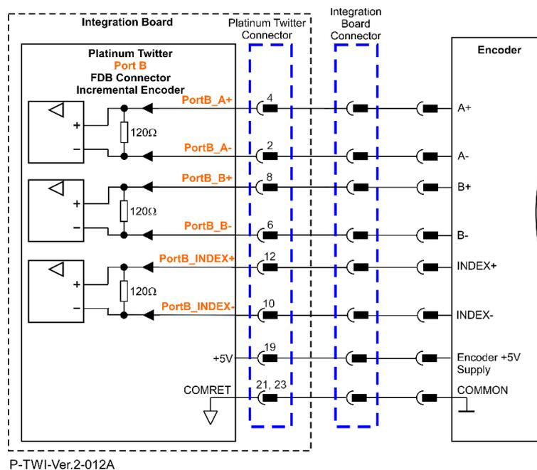
Figure 15: Port B Incremental Encoder Input – Recommended Connection Diagram
