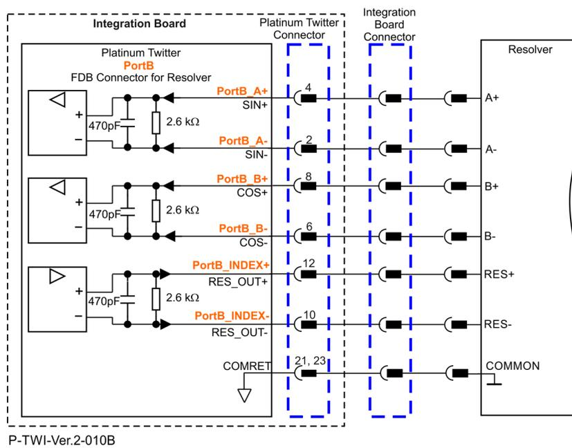
Figure 17: Port B – Resolver Connection Diagram
