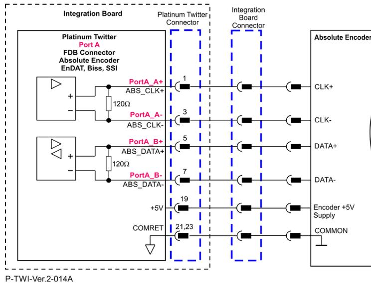
Figure 13: Absolute Serial Encoder – Recommended Connection Diagram for Endat, Biss, SSI
