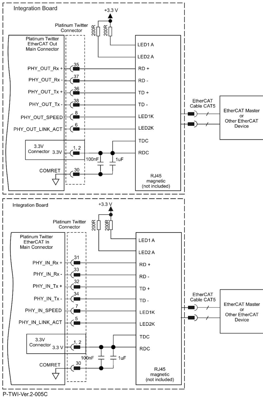
Figure 33: EtherCAT Connection Schematic Diagram
