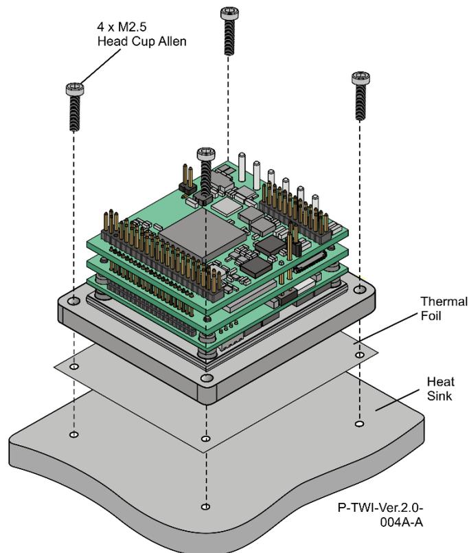
Figure 4: Mounting the Heat Sink and Thermal Foil to the Platinum Twitter
