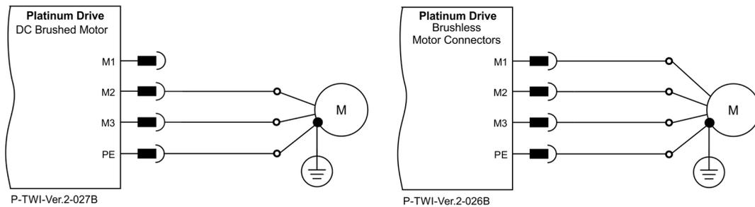
Figure 9: Brushed and Brushless Motor Power Connection Diagram
