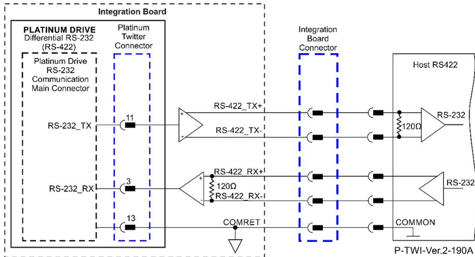
Figure 30: Differential RS-232 Communication Example
