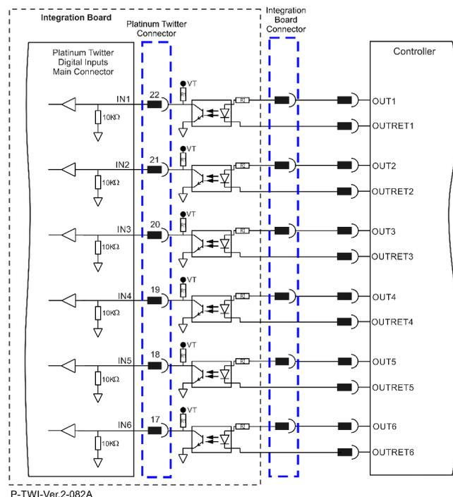
Figure 23: Digital Input 5V Logic level Mode Connection Diagram
