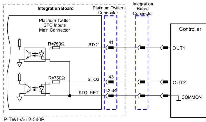
Figure 25: STO Input Connection – 5V Logic Level
