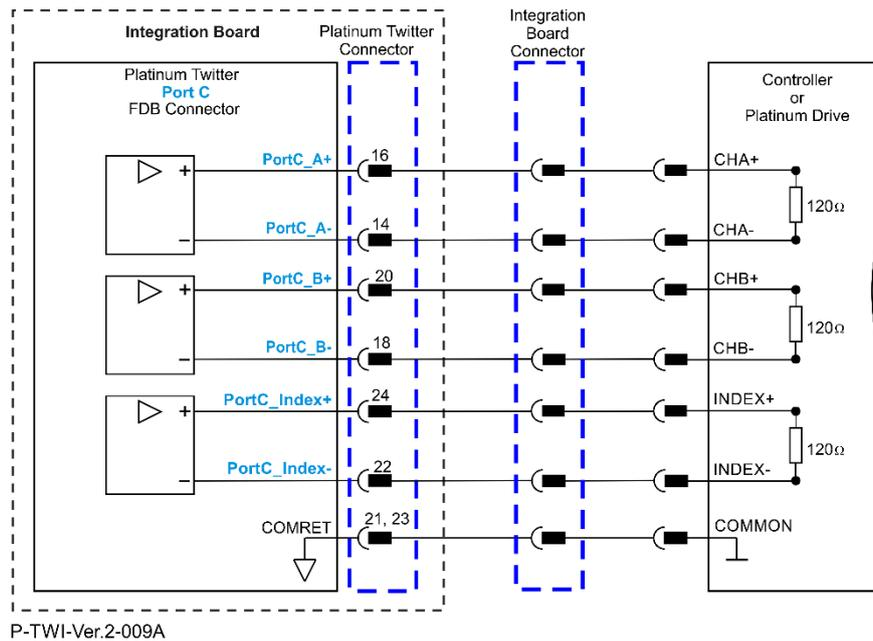
Figure 21: Emulated Encoder Differential Output – Recommended Connection Diagram
