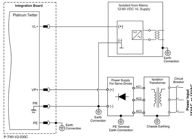
Figure 10: Ordinary Option: Separate VP and VL Power Supplies Connection Diagram
