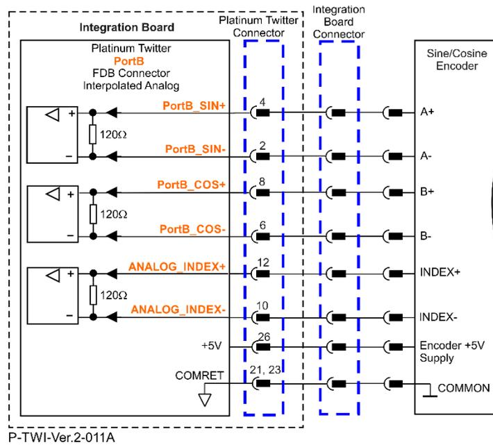
Figure 16: Port B - Interpolated Analog Encoder Connection Diagram
