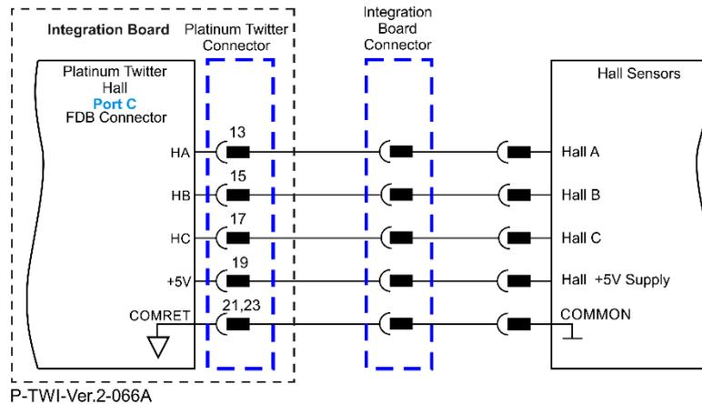
Figure 22: Hall Sensors Connection Diagram
