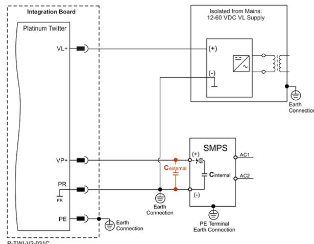
Figure 11: SMPS Option: Separate VP and VL Power Supplies Connection Diagram
