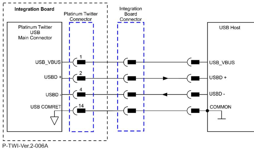
**Figure 32: USB Network Diagram**
