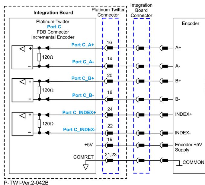
Figure 18: Port C Incremental Encoder Input – Recommended Connection Diagram
