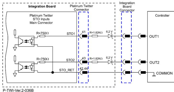
Figure 26: STO Input Connection – PLC (24V Logic)
