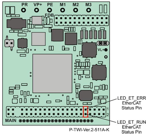
Figure 34: EtherCAT Status Indicator Pin
