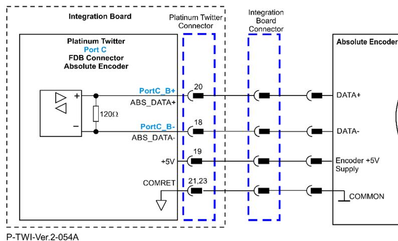
Figure 20: Absolute Serial Encoder – Recommended Connection Diagram for Panasonic, Tamagawa, Sanyo-Danki
