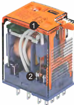
常开常闭切换后的状态 State After Switching
