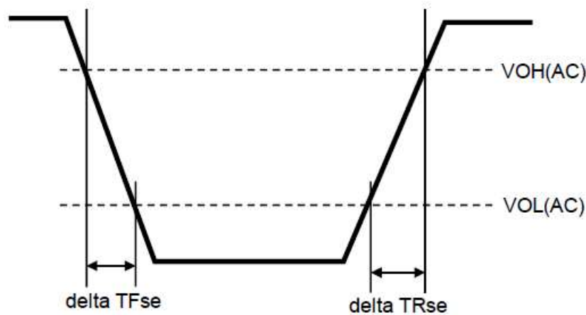
Figure 5-2. Single-ended Output Slew Rate Definition
