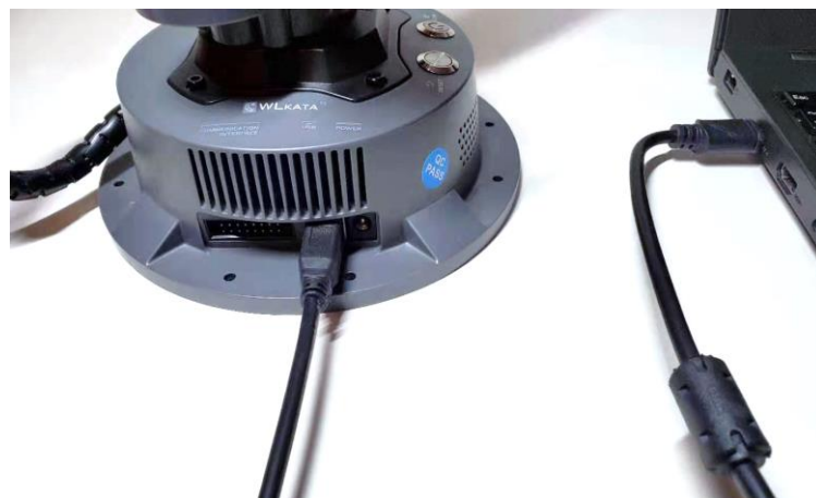
Figure 3.2 Connecting the manipulator to the computer
