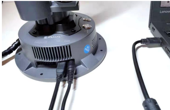
Figure 3.3 Connecting the manipulator to the power adapter
