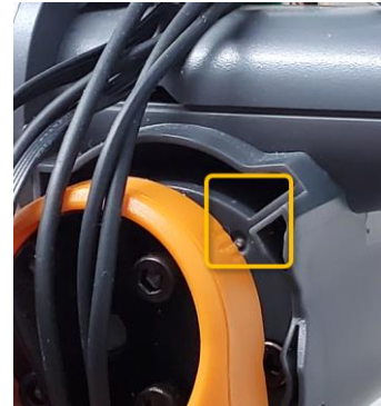
Joint 3 homing position reference
