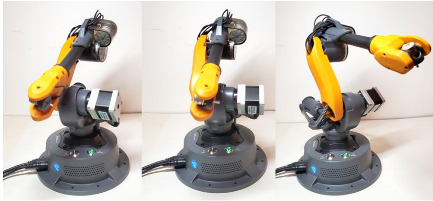
Figure 3.13 In the progress of HOMING the manipulator
