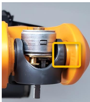
Joint 5 homing position reference
