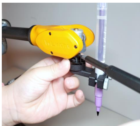
Figure 3.34 Installing the pen-holder module and the pen
