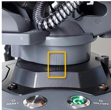
Joint 1 homing position reference
