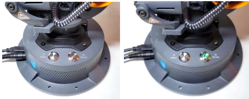
Figure 3.11 Switching on the manipulator
